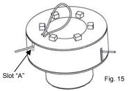
6. Pull the ends of the cutting line alternately until you have it evenly distributed through the openings.
